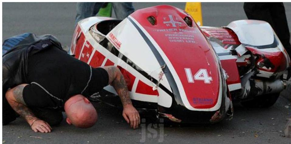
On the other hand Oscar sustained rear wheel damage, fibre glass and water pipe repairs and a bent bracket. Upon consultation with Tim Reeves solution found to rear wheel, Tommy Bennett came down to the paddock really early the next day and inspected all the welds , and Greg Lambert put off a fishing trip and got cracking at 7am with re fibre glassing Oscars main fairing and seat unit. Returning a little latter in the day to fix on brackets and fibreglass them also.
